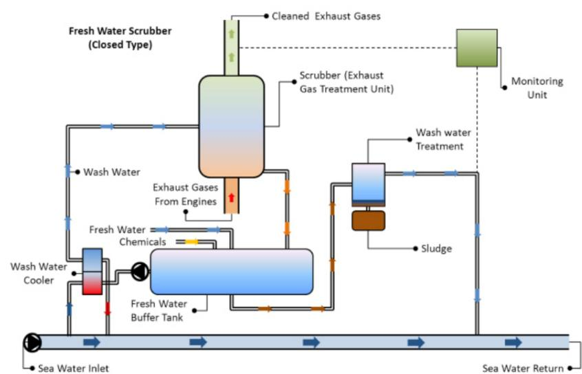
The closed type uses fresh water in “closed” fresh water circuit that is treated with an alkaline chemical such as caustic soda neutralization and scrubbing. The wash water is re-circulated and the losses is made up with additional freshwater. A small quantity of the wash water is bled off to a treatment plant before discharge to the sea. The system could also be designed with a holding tank for zero discharge for a certain period.
