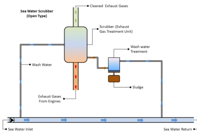
The open type uses sea water to wash the exhaust gases. The wash water is then treated and discharged back to the sea, with the natural chemical composition of the seawater being used to neutralize the results of SO<sub>2</sub> removal.
